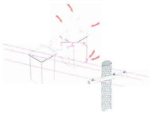
Hydraulic fluid is flammable. If electricity flows through the boom-tip, it can cause the hydraulic fluid to burn or to explode. Contact by any part of the boom-tip with an energized conductor while the boom-tip also is in contact with another energized source or a grounded object can cause the hydraulic fluid at the boom-tip to burn or explode.
